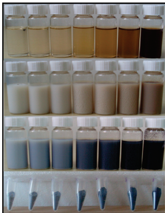
Figure 1. Sample pictures from top to bottom represent the suspensions of GO with different weight ratios dispersed in the ethanol–water solvent, suspensions of P25–GO with different addition ratios of GO before hydrothermal treatment, suspensions of P25–GR after hydrothermal treatment of P25–GO, and the final P25–GR solid product after washing, filtering, and drying process, in which, from left to right, weight addition ratios are 0.2, 0.5, 1, 2, 5, 10, and 30% GR.
